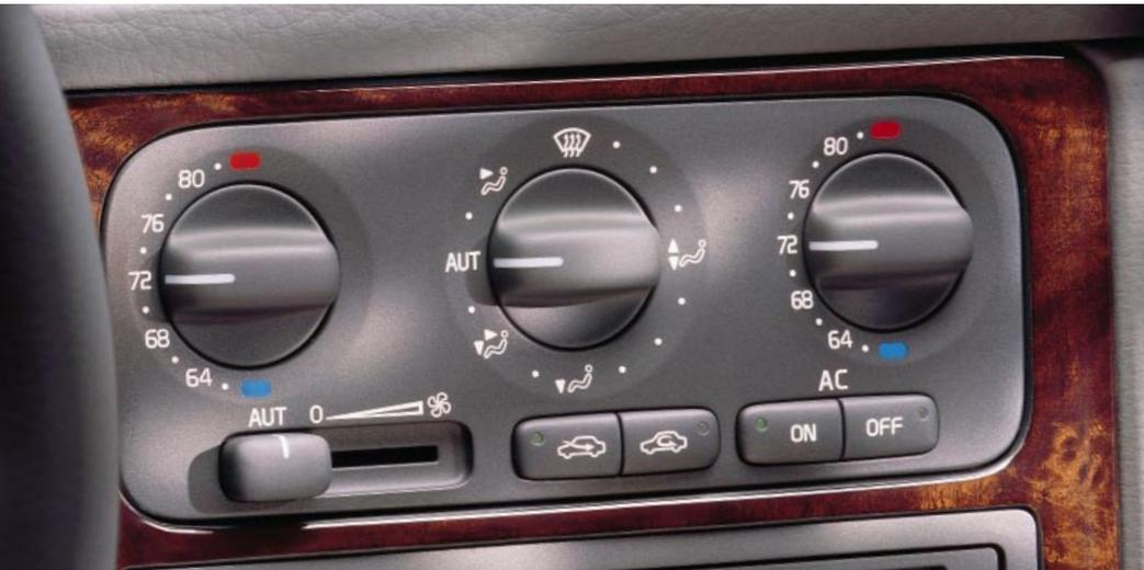
Individual temperature controls allow both driver and front seat passenger to adjust the system for their seating position. The sophisticated Electronic Climate Control system will maintain the desired individual temperature settings without further adjustment.
