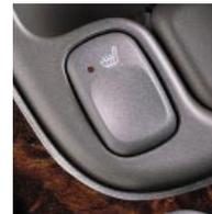
Electrically heated seating elements can be switched on to warm the seat and backrest when the interior temperature drops below 50° F (10° C).\*
