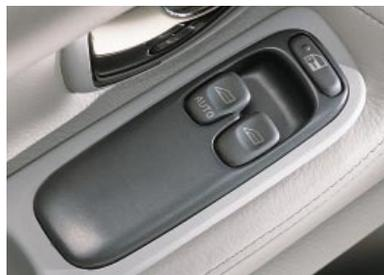
Pleasing to the touch with broad concave surfaces and a firm positive detent, switches, residing conveniently by the driver's hand, offer individual control for the windows, side mirrors and door locks.
